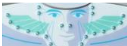
20 horizontal and vertical visual field LEDs
